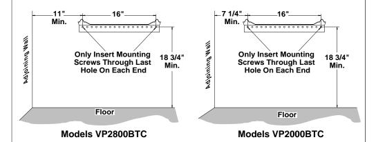
Figure 8 - Mounting Bracket Clearances
